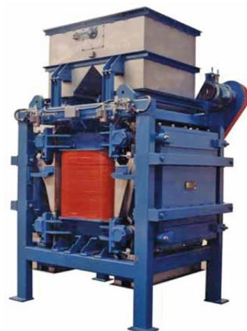
*Master Magnetics Induced Roll Separator: 1 metre width, 2 pass unit used for processing nepheline syenite.*
