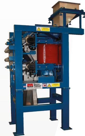
*Induced Roll Separator and control panel (500mm width, 2 roll unit)*
