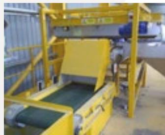
The Can Sorter ECS is a low-cost alternative to larger Eddy Current unit, for applications that do not require high specification machines.
