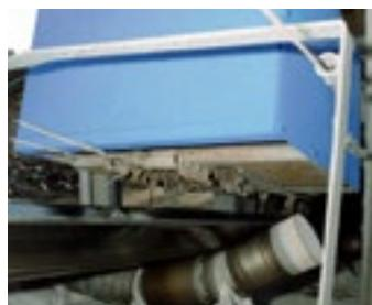
Suspension Magnets are used for the extraction of occasional tramp iron from deep product burdens. These magnetic separators are available with either a permanent magnet system or as an air-cooled or oil-cooled
