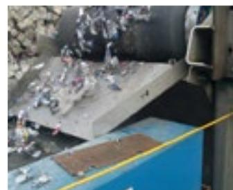
The 360° magnet system retains extracted iron, discharging it behind the centre line of the pulley, whilst the clean product follows its natural trajectory. All units are available with either ferrite or rare earth magnet systems, depending on specific extraction requirements.
